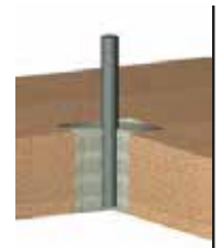
Post is installed into holes of 50x50x40cm for fixations to soil surfaces.
